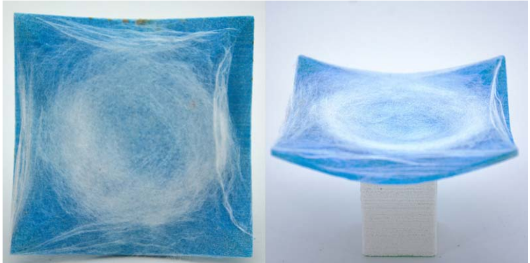
Figure 12 20mm tall thrust vault spinning platform demonstrating the silkworm's spinning behavior.
